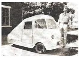
This car attracts a lot of attention wherever Gaylard Train, of Hardy, Neb., drives it. It is a three-wheeled job of his own design and construction. It uses a Model T frame which was shortened and narrowed at the rear end. It is powered by a Harley 74 and has a Harley three-speed transmission. Top speed is about 45 m.p.h. A \$3.00 Workbench check is going out to Gaylard for this snapshot.
