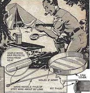
Let's make a little FRYING PAN for frying an egg at a time. It is only necessary to find the cover to one of those large cracker tins. Drill two holes about 2" apart near the top edge. Then attach about 30" of galvanized telephone wire for a handle as shown. Push the ends through the holes in the pan, turn the handle over and it will grab the pan nicely from below. Insulate the handle with wood. It can be quickly taken apart and stowed in the knapsack if camping.
