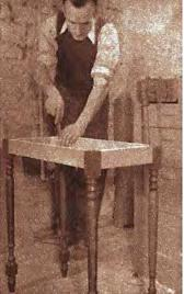
Right: Screwing the arm in place. This holds the rear top panel vertically rigid.
