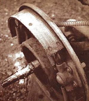
Above Left: A brake band whose action has been faked with strip of inner tube. Above Right: A brake band that has been worn down to the brass rivet heads.
