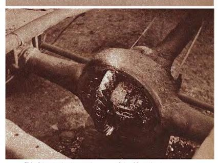
This differential has been made to run quietly with sawdust in grease.
