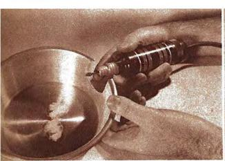
ABOVE: Gap cut into the edge of the pan makes a snug in around the top of the synchronizer battery case. RIGHT, Fitting the cut-out aluminum pan, minus reflector, in front of the flash reflector to make sure that the flash lamp isn't crowded. Black felt strip at top end of battery case makes a light-tight seal with the fitted reflector-filter unit.
