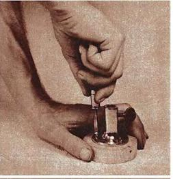
Above: Fastening flange to the wooden disc. Below: Soldering the metal "reflector" disc to the bottom of the brass-shell electrical socket (with switch removed).
