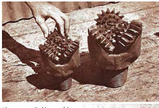
Above are rock bits, revolving grinders that are used when the going gets tough for the drill.
