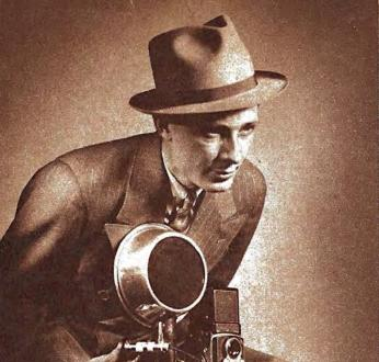
LEFT: Simple flashfilter unit clamped in front of ordinary flash reflector holds back visible rays and passes invisible infra ced. BFLOW: Taken unawares—exposed in total darkness!
